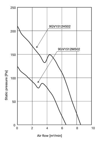
Fig. 3: Air flow vs. static pressure characteristics
