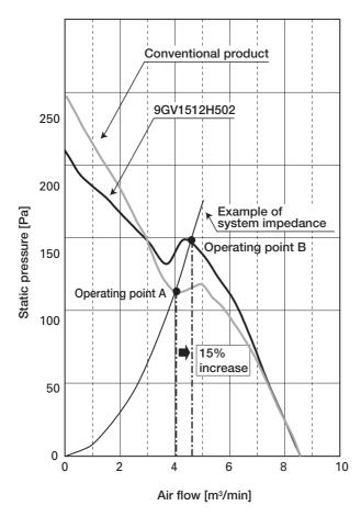
Fig. 4: Comparison of air flow vs. static pressure characteristics
