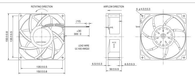
Fig. 2: Dimensions of the "San Ace 150" GV type fan
